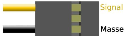
You can also use electronic sensors, e.g. inductive proximity switches from industry. These make the construction of the necessary range scanning / cam track easier. Electronic switches must be designed for 5V operating voltage and have a so-called open collector output.
