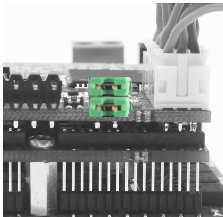
*Figure 4: do not forward BEC voltage to receiver*
