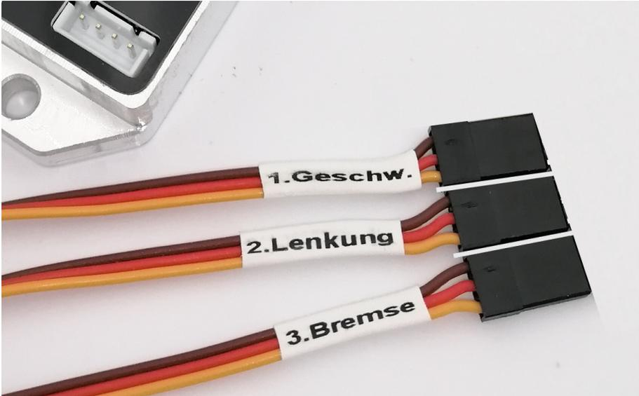
Figure 2: Control inputs. 1-throttle 2-steering 3-brake (optional usage)
