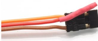
*Figure 5: Removed and insulated + supply cable in the servo plug*
