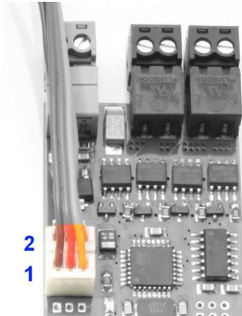
*Figure 4: Servo channel assignment*
