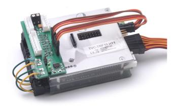
Abbildung 14: TVC-HRF-AD3 Heng Long adapter mounted on the FO module
