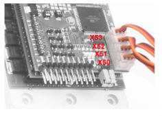
Figure 3: servo cable position
